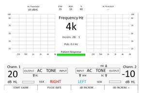
To familiarize the patient with the exam, select an increment of 4 (only for Piano) or 5 dB clicking the corresponding button on the right bottom part of the screen. Select the tone frequency and intensity (suggested value: 20 dB SL), and the pulse rate, i.e. the frequency of presentation of the occasional "jump in loudness".
